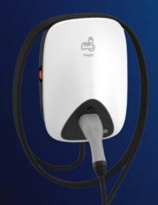
This Evlink Home product is a wall mounted charging station suitable for all electrical vehicles. The nominal output power is 7.4kW. It is supplied in single-phase (1P+N). The rated charging current is 32A under 230VAC with a 50Hz to 60Hz frequency. The charging station is easy to install (no special tools required). It is recommended for private use at home.
